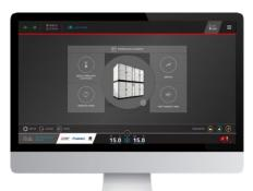
With a simple Ethernet connection, it is possible to connect KIPlink to the facility LAN and get full access to the unit's control with a browser. Through a VPN it is also possible to access the menu from anywhere that has an Internet connection.
